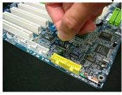
3. Connect front USB cable to the M/B pin connector according to its pin assignment.
