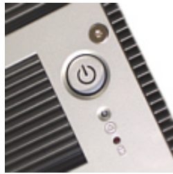
On/Off Button with LED
